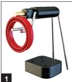
1 Fix the handle in the stand hole then put two arms inside the seal.
