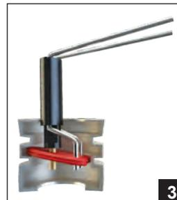
3 Hold the handles, then put the seal into the gland hold carefully.
