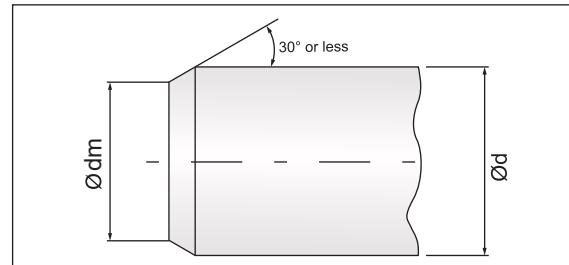
Fig. 6 : Shaft lead-in chamfer
