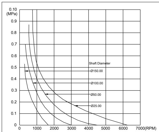
Fig. 8 : Permissible overpressure.
