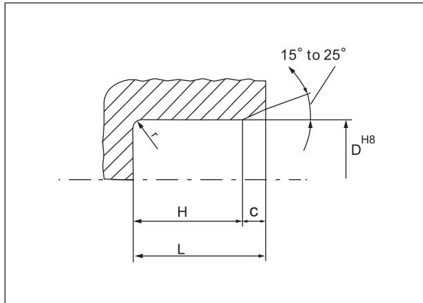
Fig. 9 : Housing drawing with depth and chamfer.
