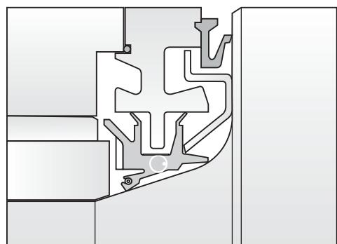
Neck seals primary shaft seal for oil film bearing used in back-up rolls or rolling mills (cold and hot). Seals oil inside and water outside by fixing the inner surface to the shaft (roll) and sliding two sealing lips on the housing side against the housing.
