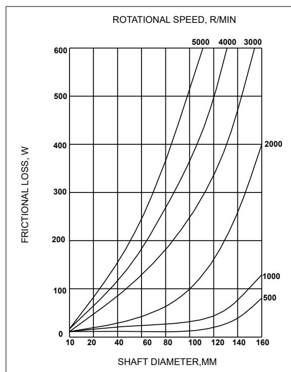
Fig. 7 : Frictional loss for standard NBR oil seal
