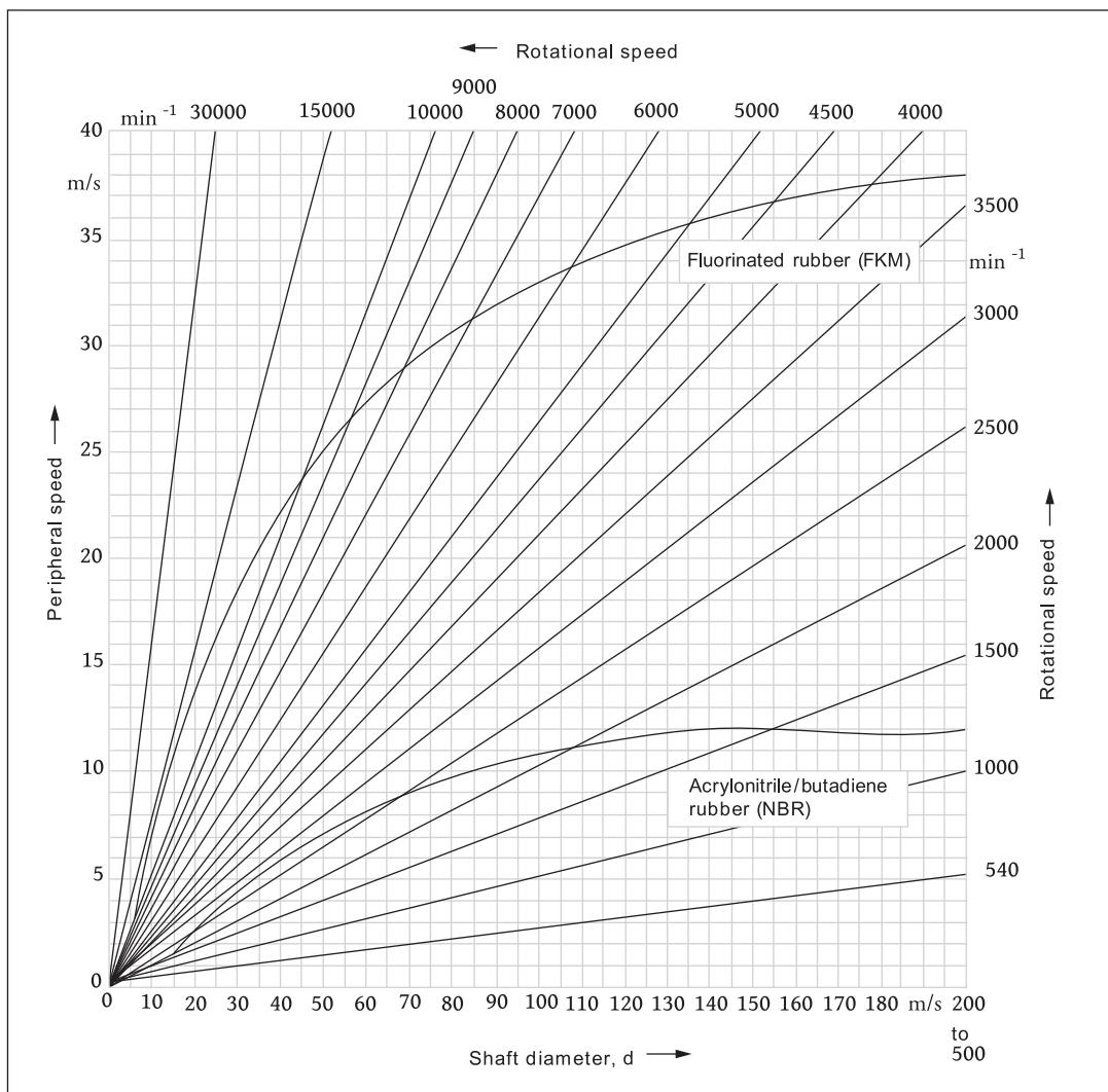
Fig. 5 : Maximum permissible rotational speed for unpressurised operation.
